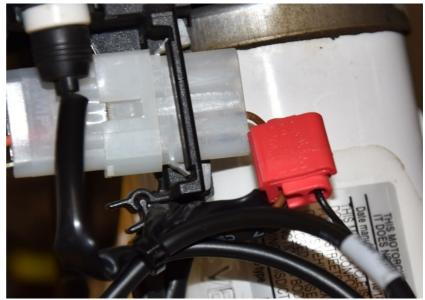
Connect GPX Red wire to the FI warning lamp connector Orange wire.
