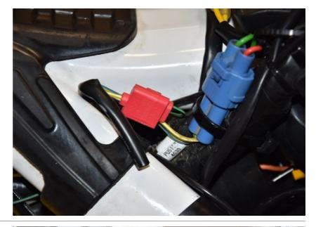
Connect the 3-pole sensor connector to the GPX wiring harness connector and coil up the excess length.
